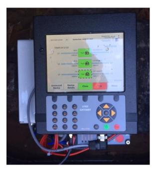
The Lynx communicates with the Gateway device (Figure 4), which provides a remote connection to the installed devices. This enables remote monitoring and control via the NMS. Figure 5 shows a typical Weezap and Lynx configuration on Smart Street including the connectivity.
