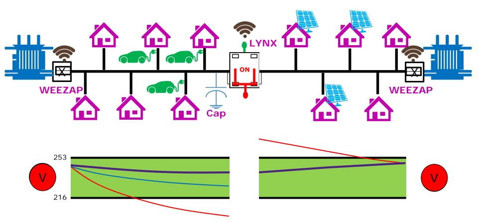
Capacitors help to bring back V in highly loaded feeders
