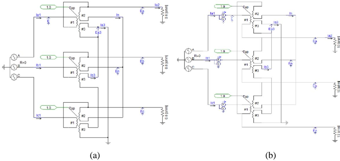
Figure 19: Equivalent PSCAD model of pP+ for voltage step down and boost function
