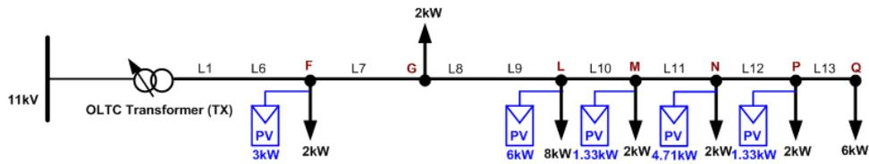
Figure 28: Single line study with PV connection
