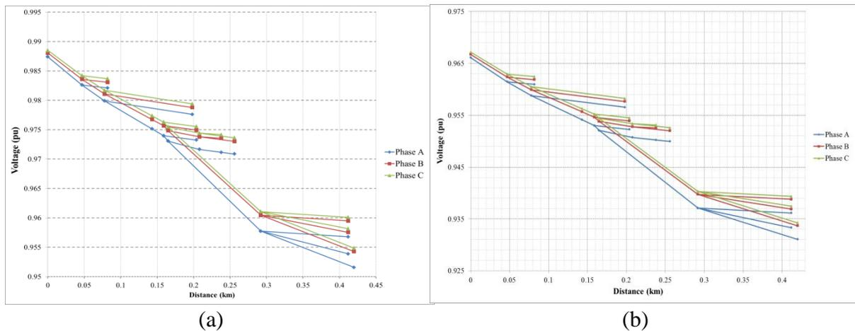
Figure 7: Voltage profile of unity tap (a) vs. -2.2% tap at Leicester Av feeder 260055783 (b)
