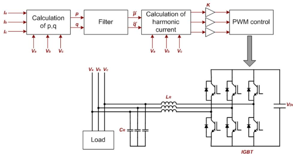
Figure 1: Control algorithm of active filter model
