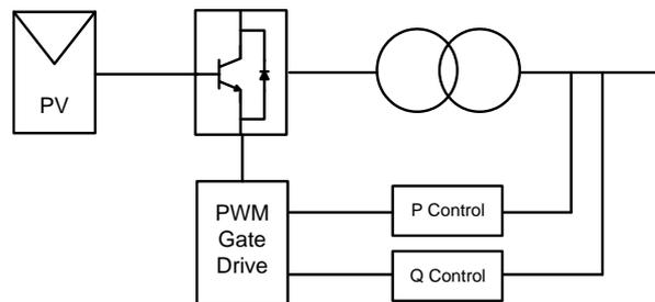
Figure 24: PV system schematic
