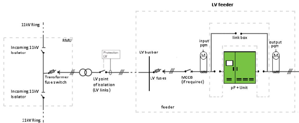
Figure 21: powerPerfactor unit feeder connection
