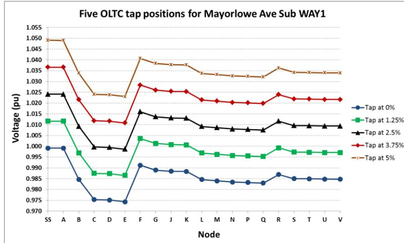
Figure 10: Voltage profile of different tap positions (unity load power factor)
