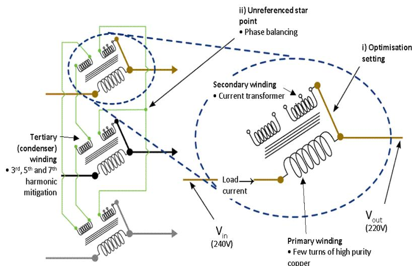
Figure 16: powerPerfector winding configuration
