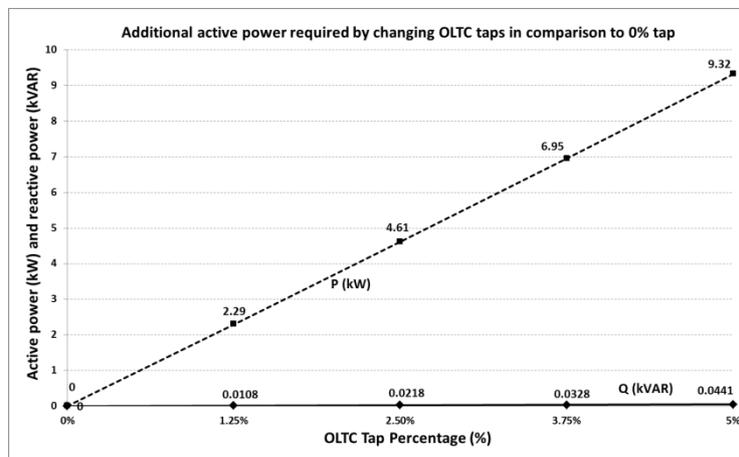
Figure 14: Additional P and Q from grid to LV feeder vs. OLTC tap positions
