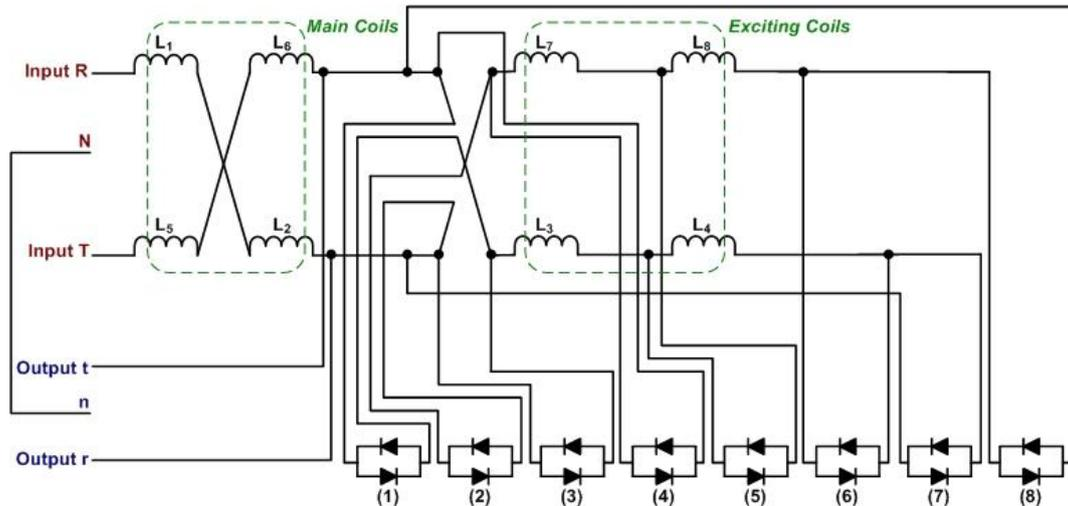
Figure 17: Two winding schematic of a pP unit operation
