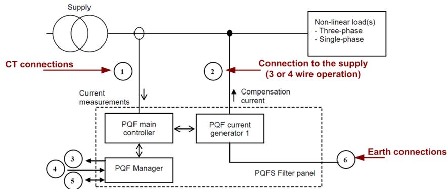
Figure 3: ABB active filter PQFS schematic
