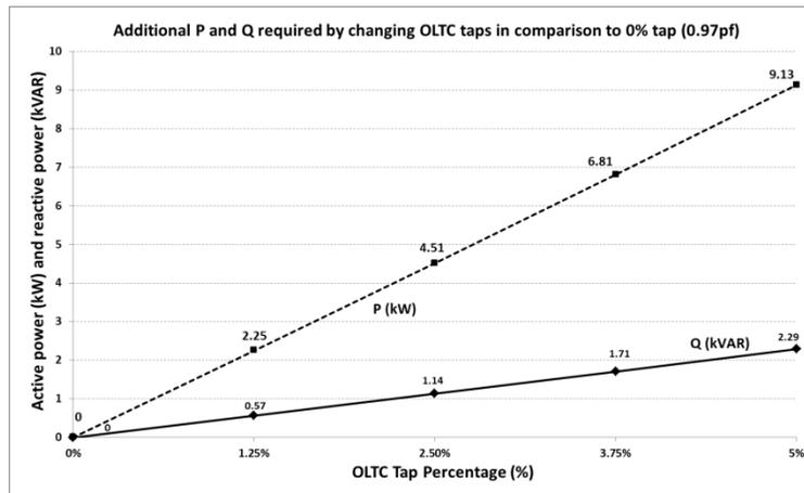
Figure 15: Additional P and Q from grid to LV feeder vs. OLTC tap positions (0.97pf)
