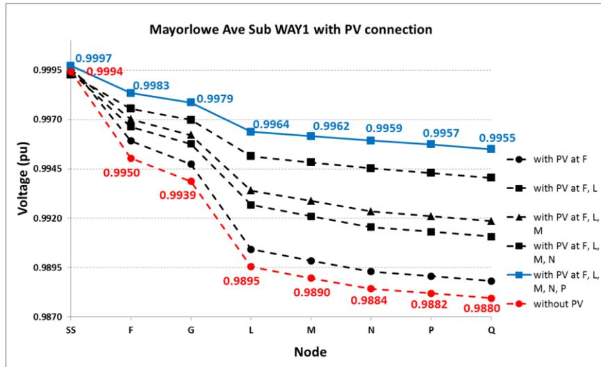
Figure 29: Effect of PV on single line
