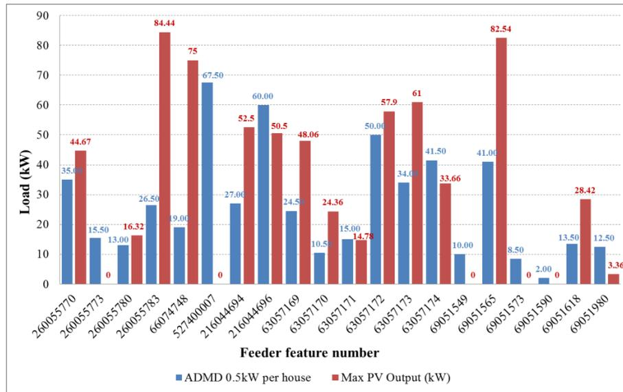
Figure 33: Total PV rating and load demand of all feeders
