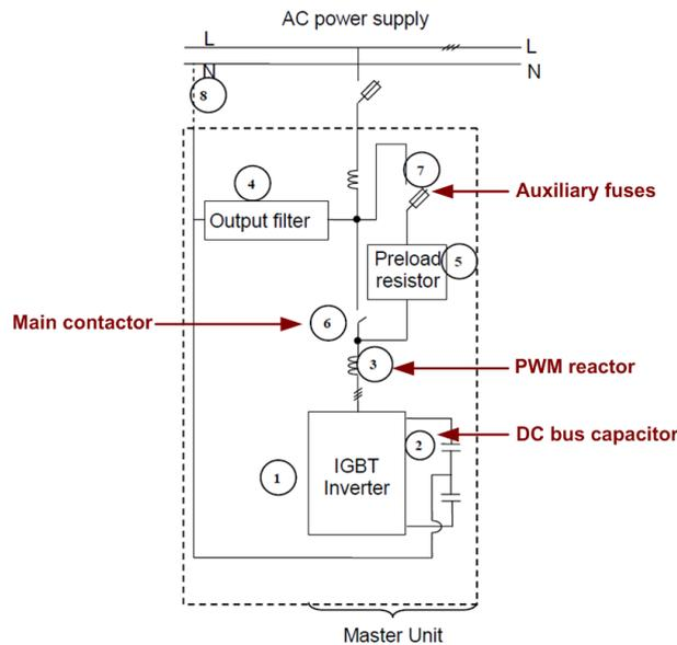
Figure 4: ABB active filter PQFS
