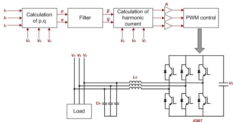
Figure 5: Control algorithm of active filter model
