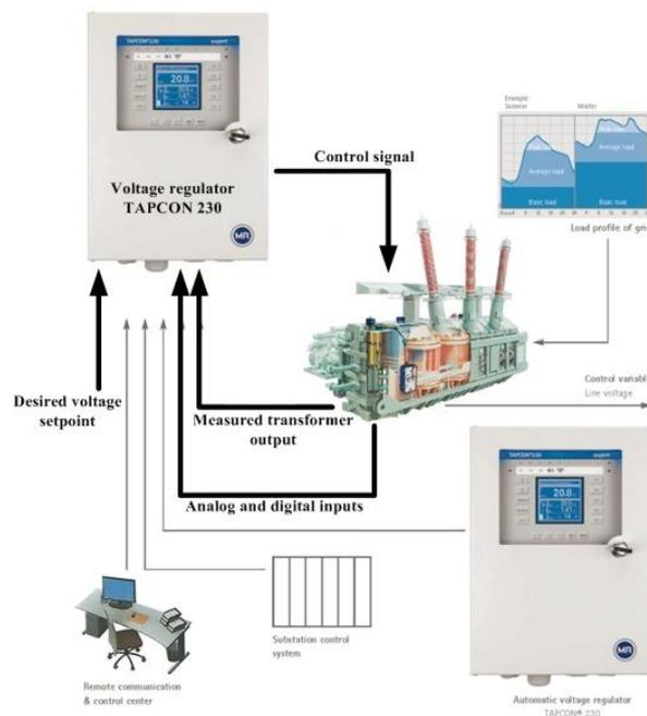
Figure 6: Overview of TAPCON voltage regulator
