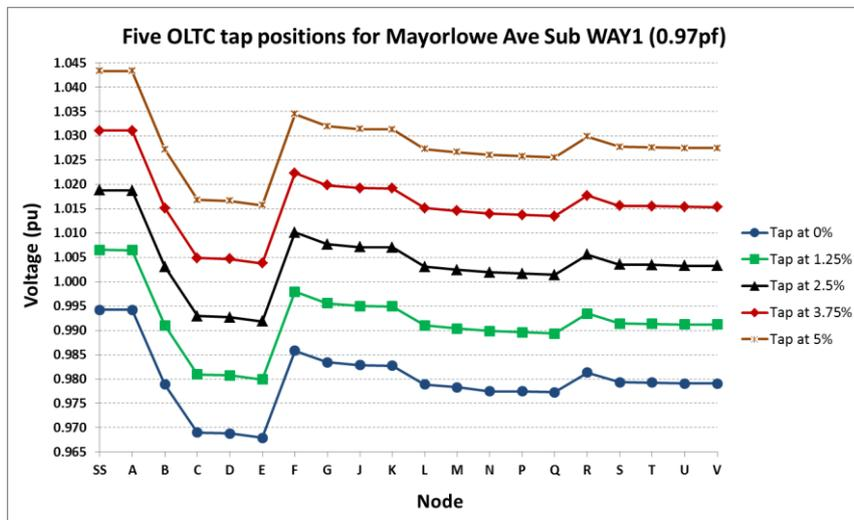
Figure 12: Voltage profile of different tap positions (0.97 load power factor)
