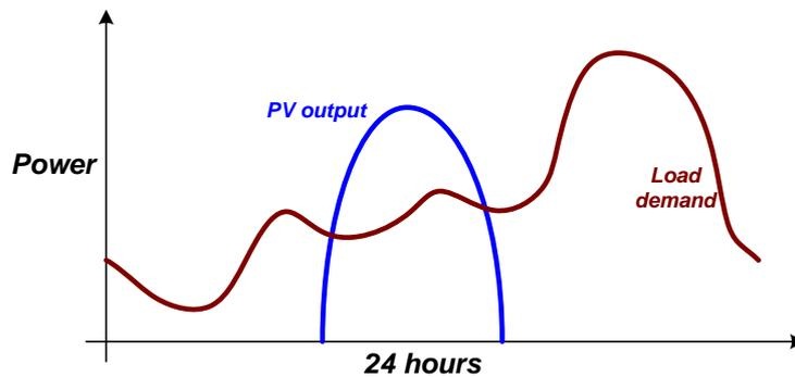
Figure 31: Theoretical PV generation and load matching profile
