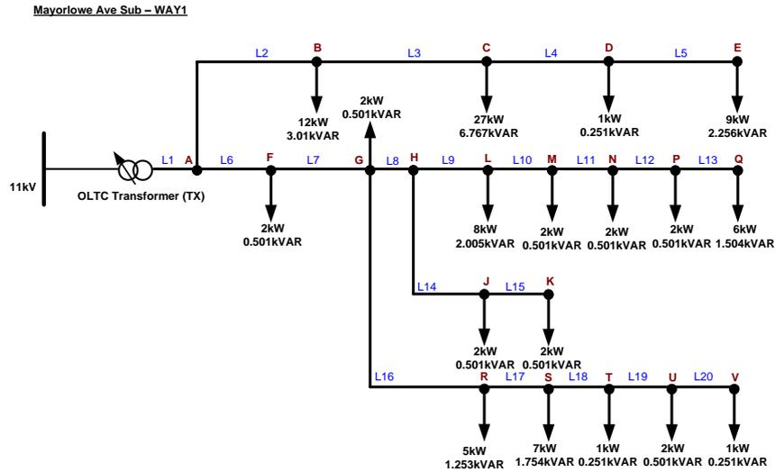
Figure 11: Mayorlowe Ave Sub – WAY1 simulation model (0.97 load pf)
