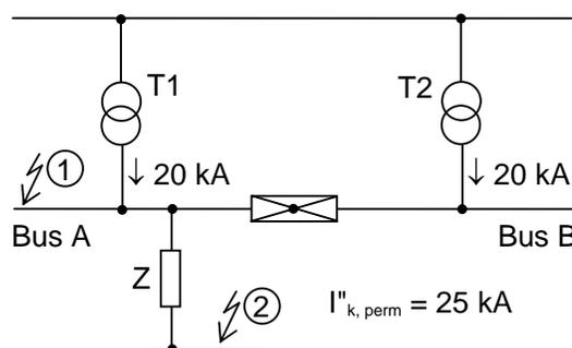
Figure 2: Example for calculation of the Tripping Values
