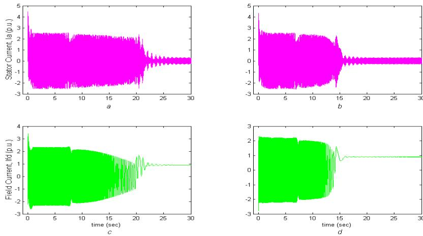
**Figure 6-6: Stator and rotor current for direct on line acceleration of SG:**
