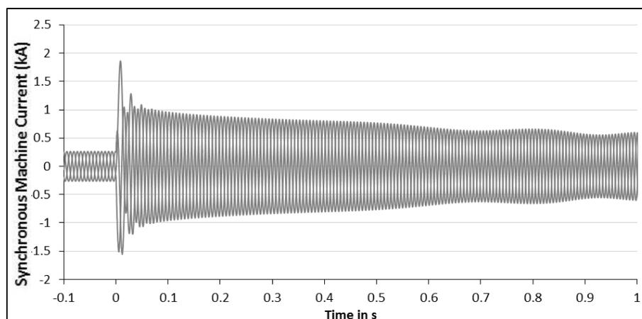
Figure 4-1: Three phase synchronous generator current during a 1 s fault.
