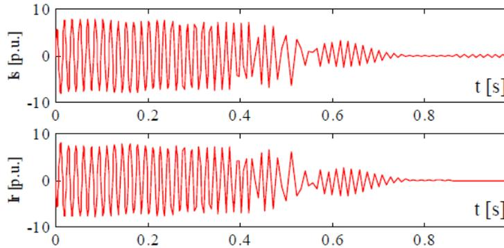
Figure 6-3: Stator and rotor current of IM during acceleration from stand still
