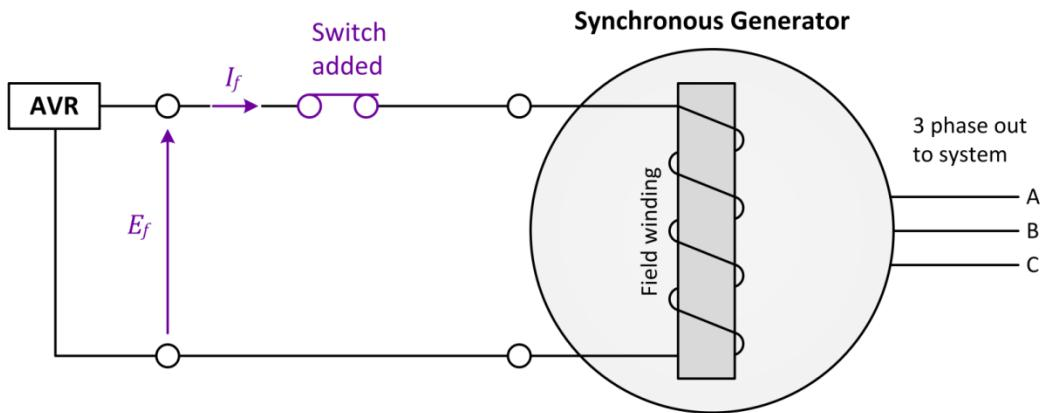
Figure 3-5: Passive flux discharge diagram for synchronous machine.
