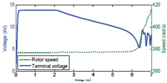
Figure 6-2: Rotor speed and terminal voltage of generator following loss of excitation.
