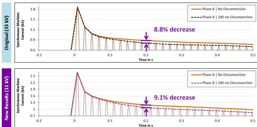
**Figure 4-12: Generator currents with excitation disconnection for original network and reconfigured with fault on 11 kV bus – phase B extreme positive values, 0–500 ms.**
