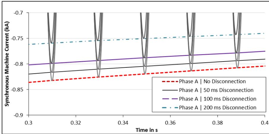
**Figure 4-8: Generator currents with excitation disconnection – phase A extreme positive values, 300–400 ms.**
