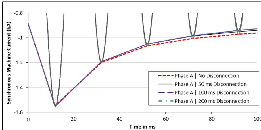
Figure 4-6: Generator currents with excitation disconnection – phase A extreme negative values, 0–100 ms.
