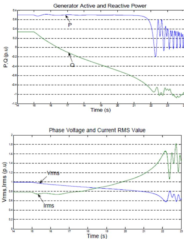
**Figure 6-1: Real and reactive power and voltage and current of generator following loss of excitation.**
