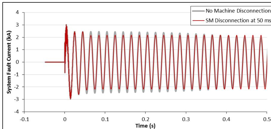
Figure 4-23: Synchronous machine disconnection – current at fault location.
