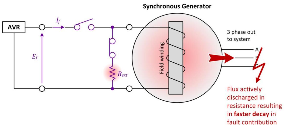
Figure 3-10: Active flux discharge – flux discharges in external resistance during fault.
