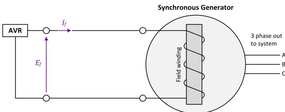
Figure 3-1: Standard excitation of a synchronous machine.
