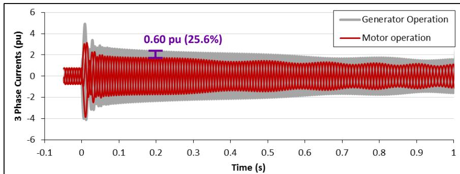
Figure 4-25: Synchronous machine operated as a motor – machine currents.
