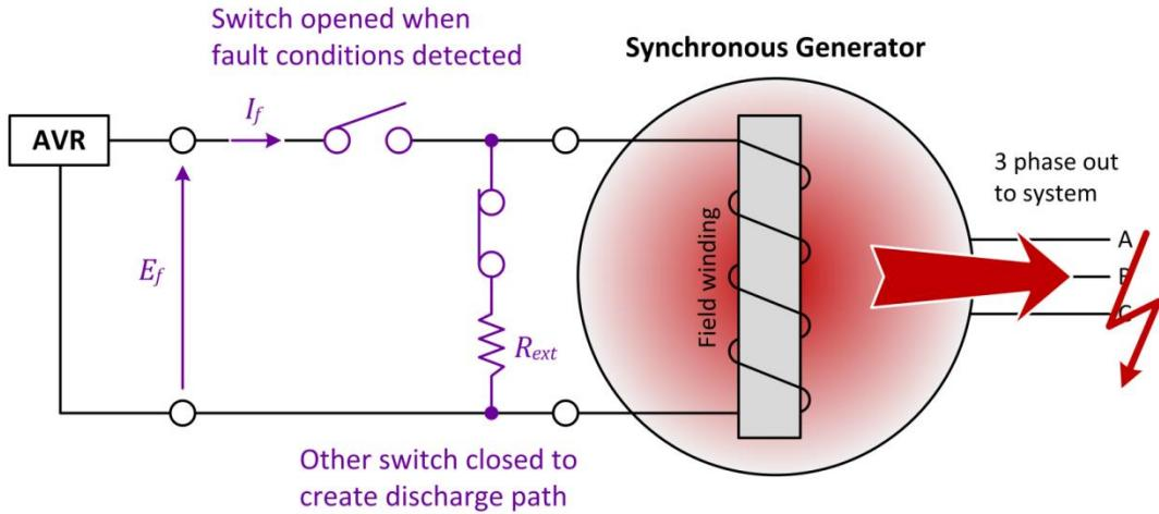
Figure 3-9: Active flux discharge – switches operate when fault is detected.
