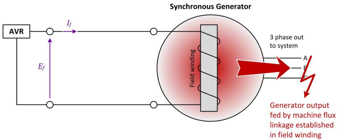
Figure 3-3: Standard excitation – feeding the fault.
