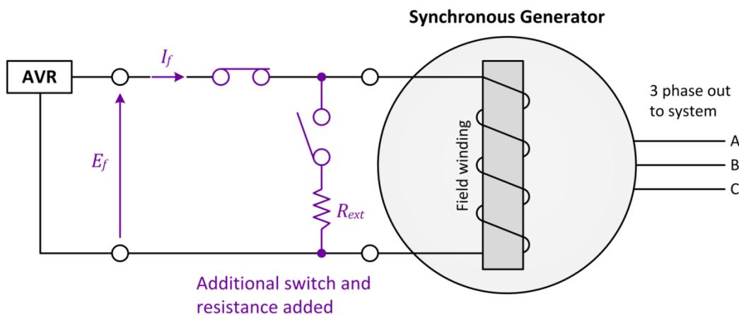
Figure 3-8: Active flux discharge diagram for synchronous machine.
