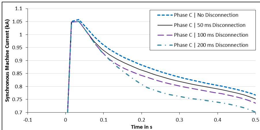
Figure 4-10: Generator currents with excitation disconnection – phase C extreme positive values, 0–500 ms.
