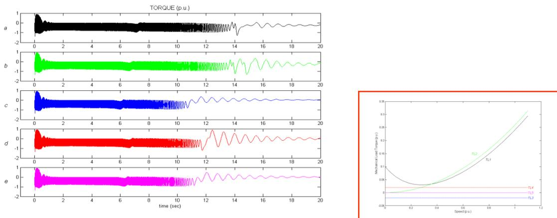
**Figure 6-7: Acceleration of SG with different load torque**
