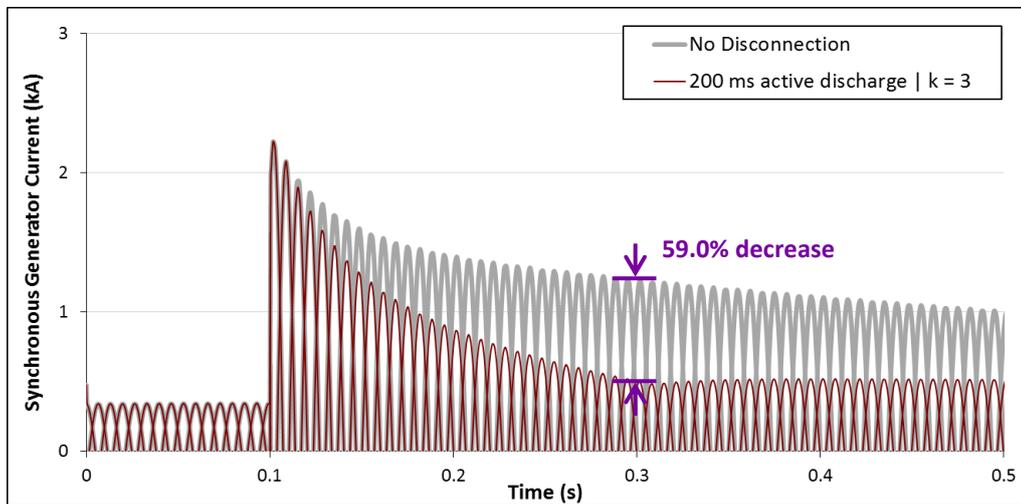
Figure 4-18: Simplified generator model – active flux discharge,  $k = 3$ .
