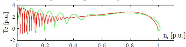
Figure 6-4: Electromagnetic torque of IM during acceleration from stand still with different inertia constants (green  $H=0.2$ , red  $H=0.07$ )
