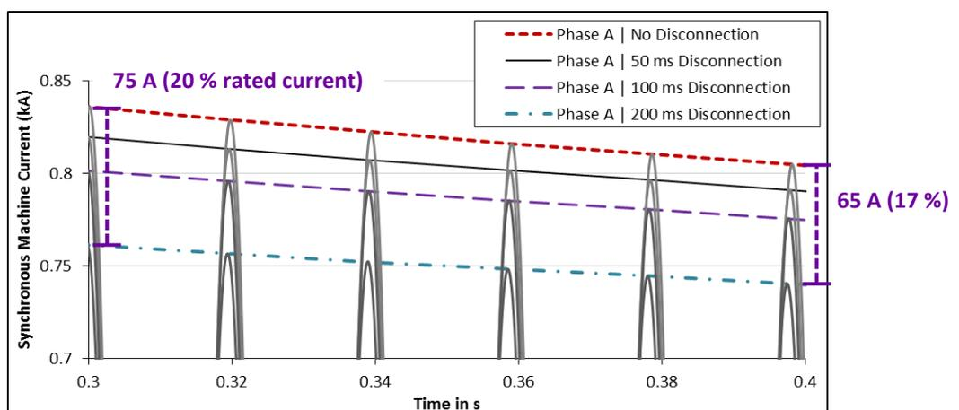
Figure 4-7: Generator currents with excitation disconnection – phase A extreme positive values, 300–400 ms.
