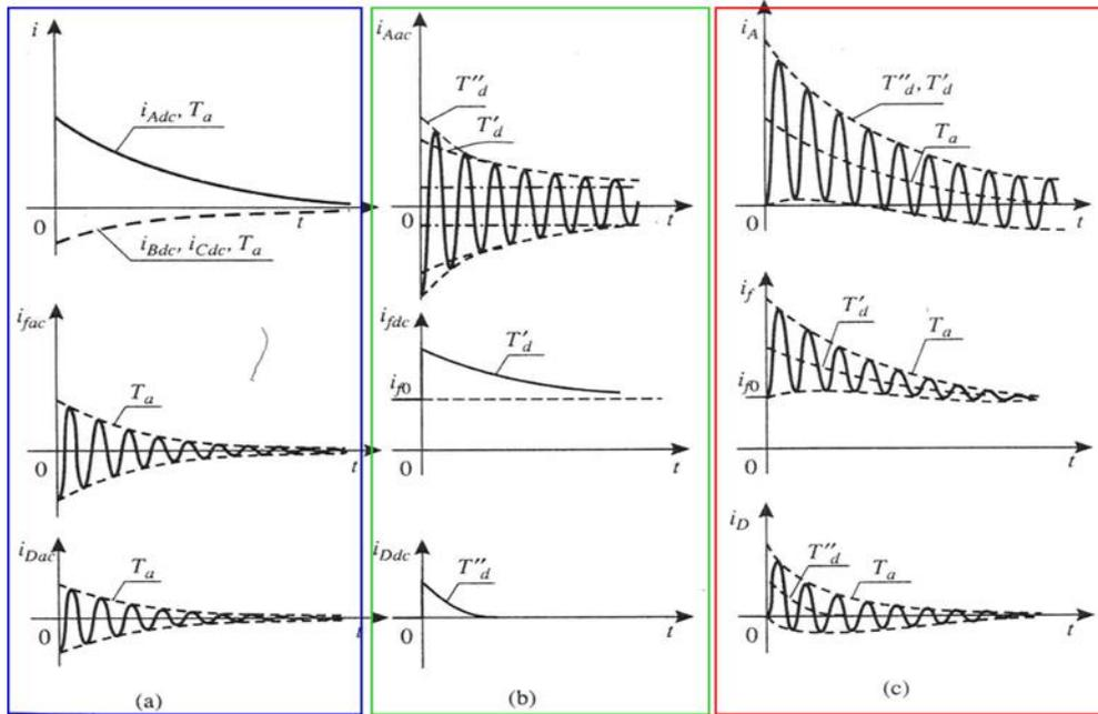
Short-circuit currents in the generator: (a) dc component of the phase current and the corresponding ac component of the field and damper winding current; (b) ac component of the current in phase A and the corresponding dc component of the field and damper winding current; (c) the resulting current in phase A, the field and the damper winding as the sum of the currents shown in (a) and (b)
