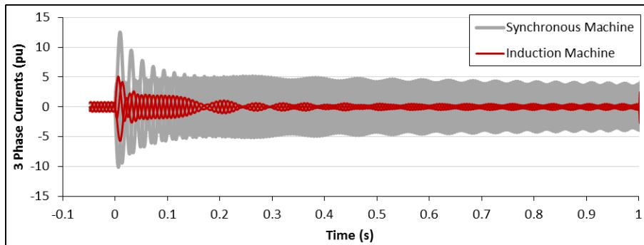
**Figure 4-20: Comparing synchronous and induction machines – three phase currents.**
