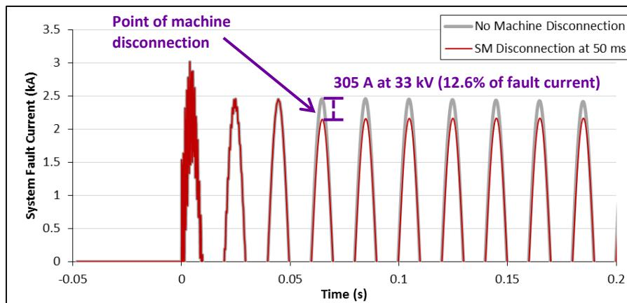
Figure 4-24: Synchronous machine disconnection – current at fault location (zoomed plot).
