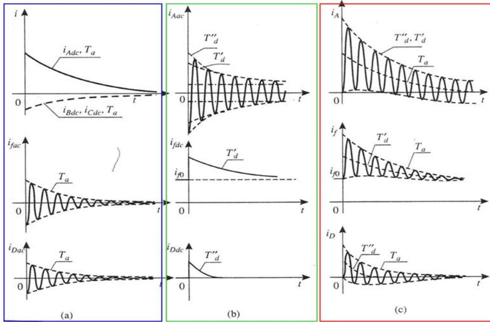
Short-circuit currents in the generator: (a) dc component of the phase current and the corresponding ac component of the field and damper winding current; (b) ac component of the current in phase A and the corresponding dc component of the field and damper winding current; (c) the resulting current in phase A, the field and the damper winding as the sum of the currents shown in (a) and (b)
