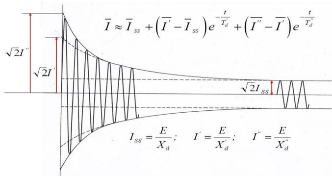
Figure 6-9: Symmetrical fault current induced in one phase of generator (no dc-offset)
