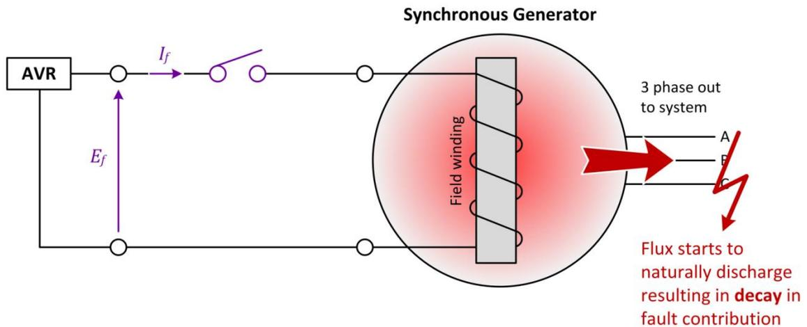
Figure 3-7: Passive flux discharge – flux discharges during fault.
