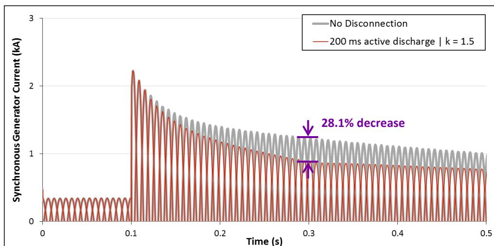
Figure 4-16: Simplified generator model – active flux discharge,  $k = 1.5$ .
