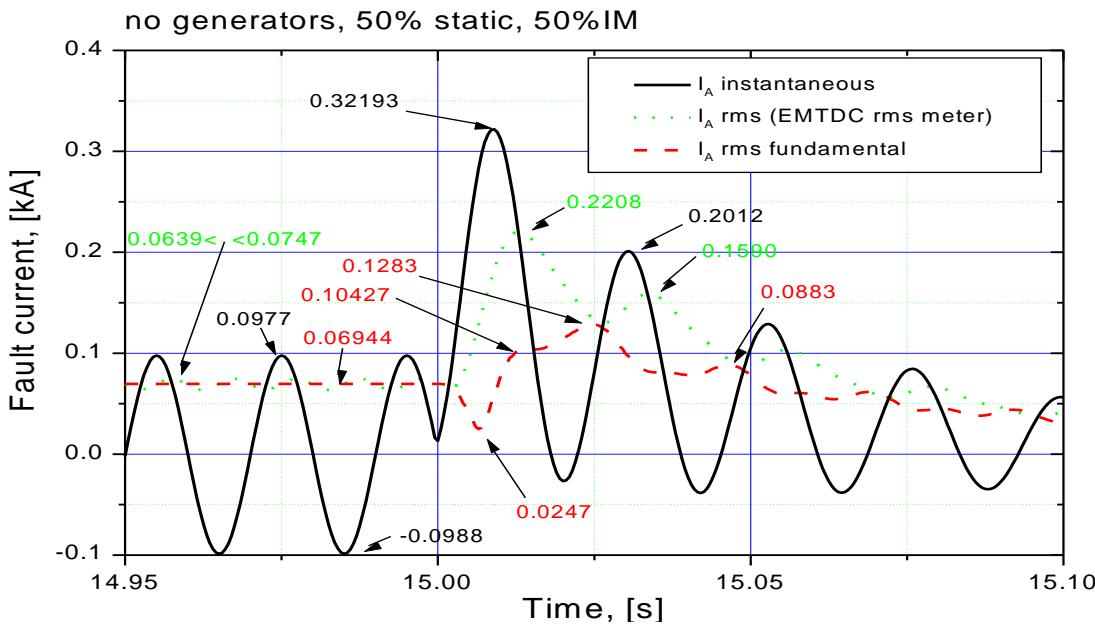
**Figure 6-12: Fault current contribution by aggregate load without generators considering different estimation methods**
