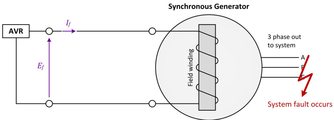
Figure 3-2: Standard excitation – a fault occurs.
