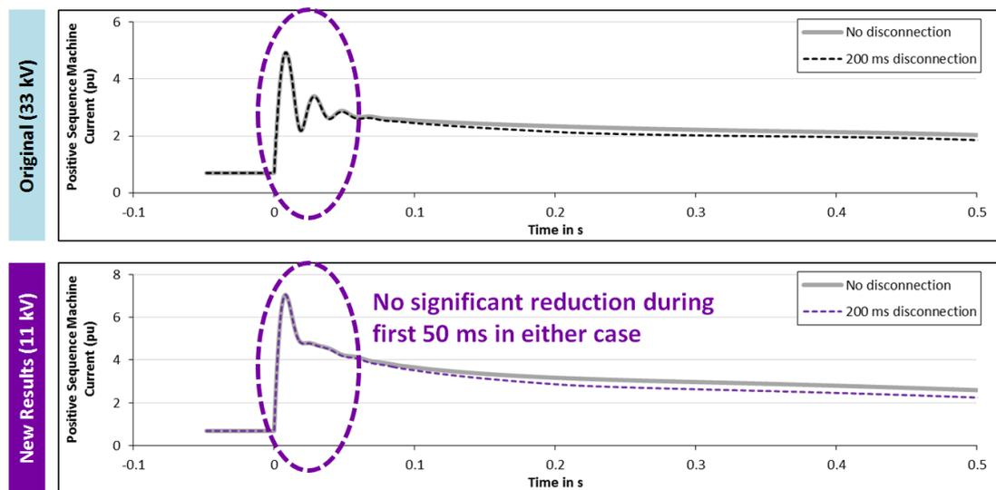
**Figure 4-13: Generator positive sequence current with excitation disconnection for original network and reconfigured with fault on 11 kV bus, 0–500 ms.**
