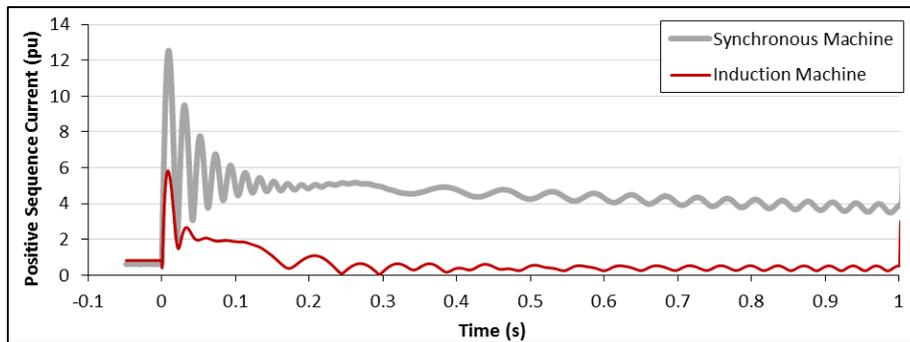
Figure 4-21: Comparing synchronous and induction machines – positive sequence currents.
