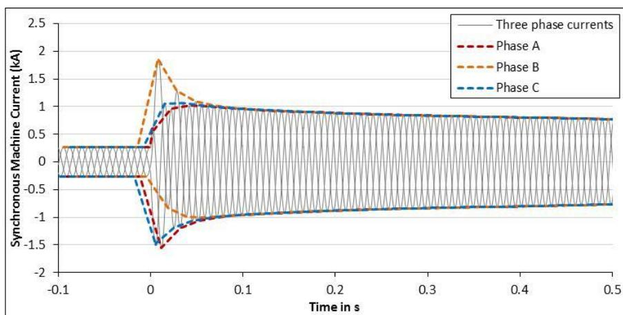
Figure 4-2: Generator currents with no disconnection – zoom of first 500 ms.
