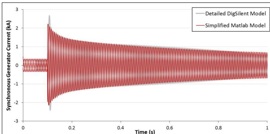
Figure 4-14: Validation of simplified Matlab generator model against detailed DiGILENT model.
