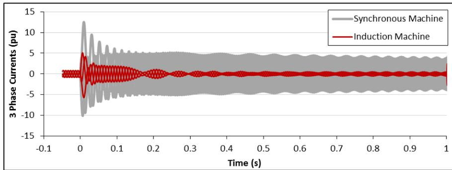
Figure 4-20: Comparing synchronous and induction machines – three phase currents.
