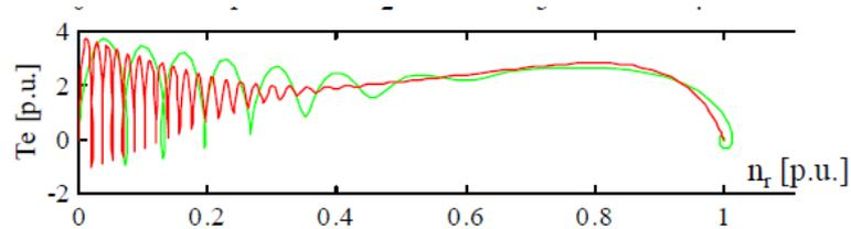
Figure 6-4: Electromagnetic torque of IM during acceleration from stand still with different inertia constants (green H=0.2, red H=07)
