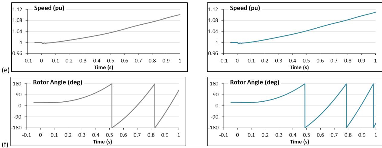
**Figure 4-4: Generator outputs during three phase network fault with no disconnection and with 200 ms disconnection of the excitation voltage. Parameters shown are (a) terminal voltage, (b) active power, (c) excitation voltage, (d) excitation current, (e) speed, and (f) rotor angle.**
