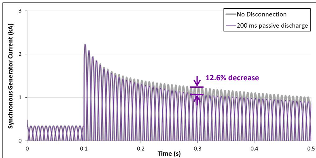
Figure 4-15: Simplified generator model - passive flux discharge.
