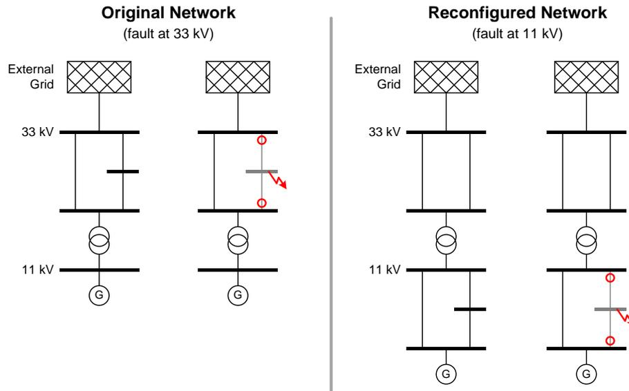
Figure 4-11: Network models for the original system and the reconfigured '11 kV fault' system.
