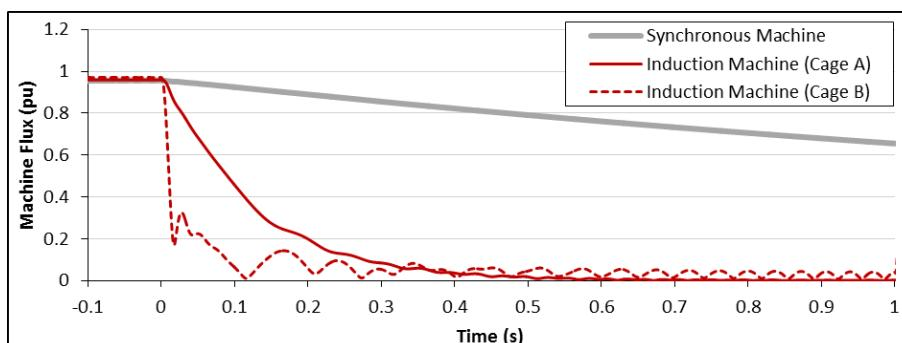
**Figure 4-22: Comparing synchronous and induction machines – machine flux.**
