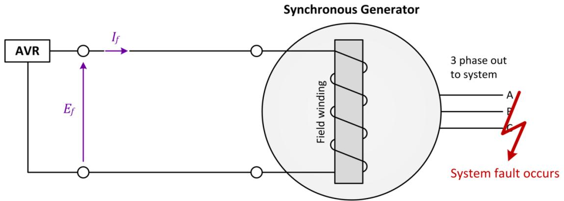
Figure 3-2: Standard excitation – a fault occurs.
