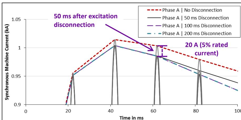
**Figure 4-5: Generator currents with excitation disconnection – phase A extreme positive values, 0–100 ms.**
