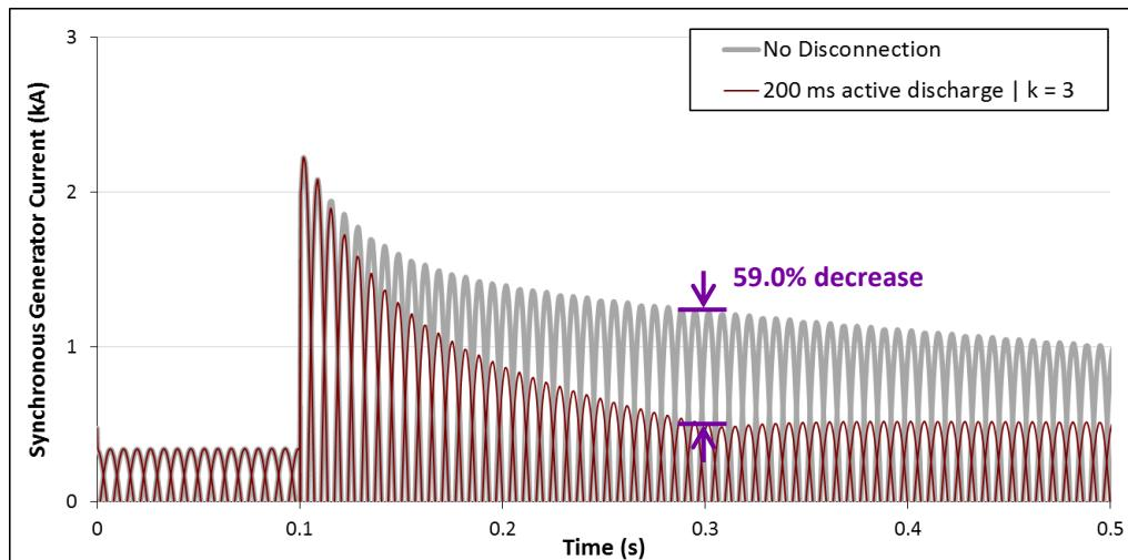
Figure 4-18: Simplified generator model – active flux discharge,  $k = 3$ .
