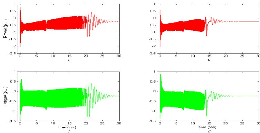
Figure 6-5: Power and torque traces for direct on line acceleration of SG:
