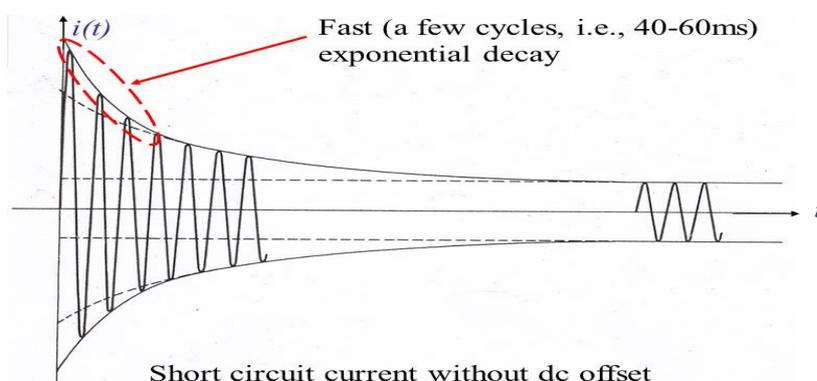
Figure 6-11: Duration of subtransient current induced in one phase of generator (no dc-offset)
