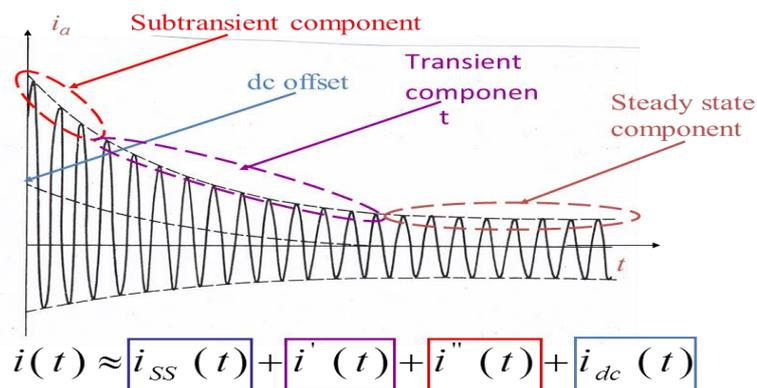
Figure 6-10: Asymmetrical fault current induced in one phase of generator – with different current components
