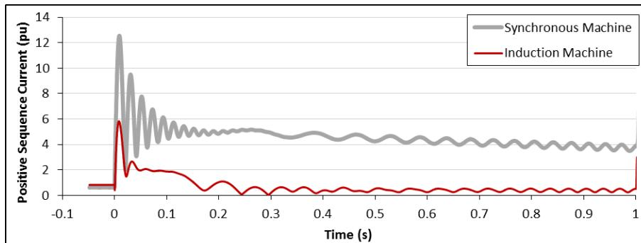
**Figure 4-21: Comparing synchronous and induction machines – positive sequence currents.**
