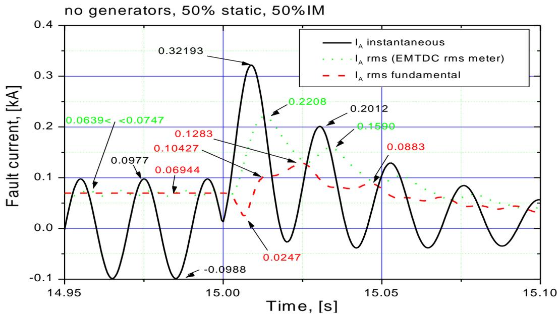
Figure 6-12: Fault current contribution by aggregate load without generators considering different estimation methods
