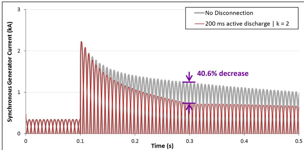
Figure 4-17: Simplified generator model – active flux discharge,  $k = 2$ .
