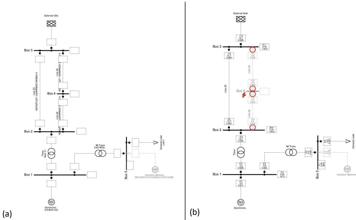
Figure 2-1: Network model shown (a) during normal operation, and (b) following a fault at bus 4.
