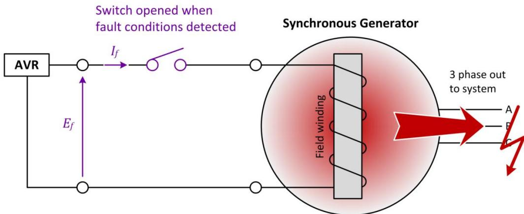
Figure 3-6: Passive flux discharge – switch opens when fault is detected.
