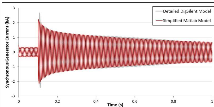
Figure 4-14: Validation of simplified Matlab generator model against detailed DigSILENT model.
