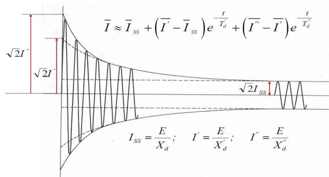
**Figure 6-9: Symmetrical fault current induced in one phase of generator (no dc-offset)**
