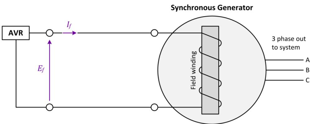
Figure 3-1: Standard excitation of a synchronous machine.
