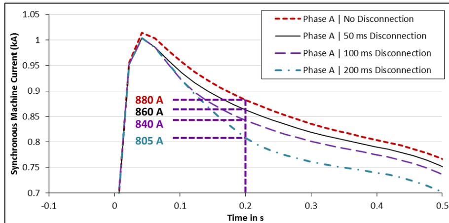
Figure 4-3: Generator currents with varying lengths of excitation disconnection – phase A extreme positive values.
