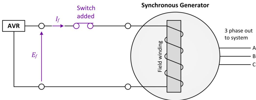
Figure 3-5: Passive flux discharge diagram for synchronous machine.
