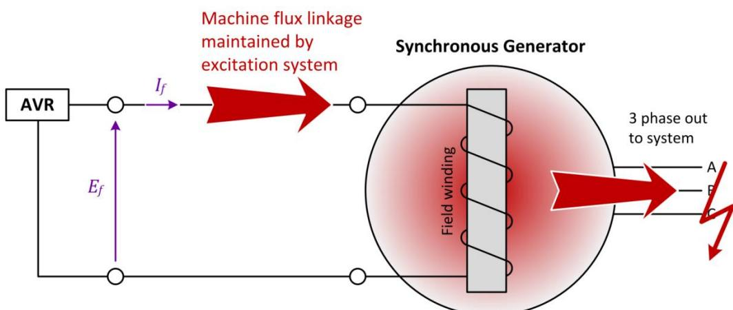
Figure 3-4: Standard excitation – maintaining the machine flux linkage.
