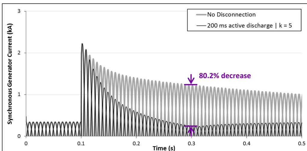
Figure 4-19: Simplified generator model – active flux discharge,  $k = 5$ .
