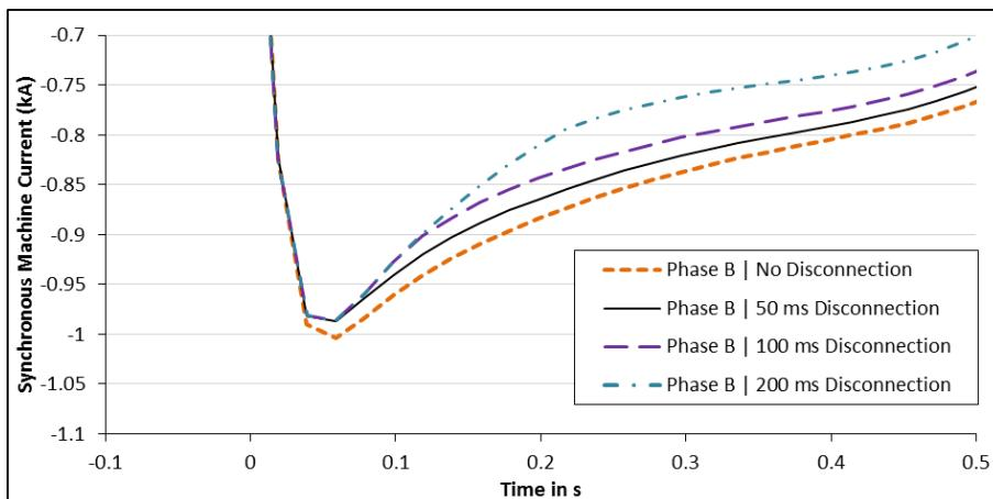
**Figure 4-9: Generator currents with excitation disconnection – phase B extreme negative values, 0–500 ms.**
