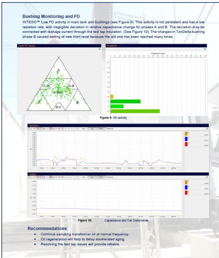
Figure 3: Bushing monitoring and partial discharge
