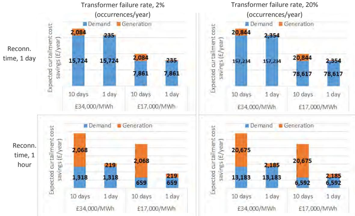
Figure 5.2: Savings in curtailments costs from installing a third transformer
