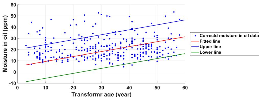
Figure 3.5: Fitting of moisture in oil data of outdoor distribution transformers
