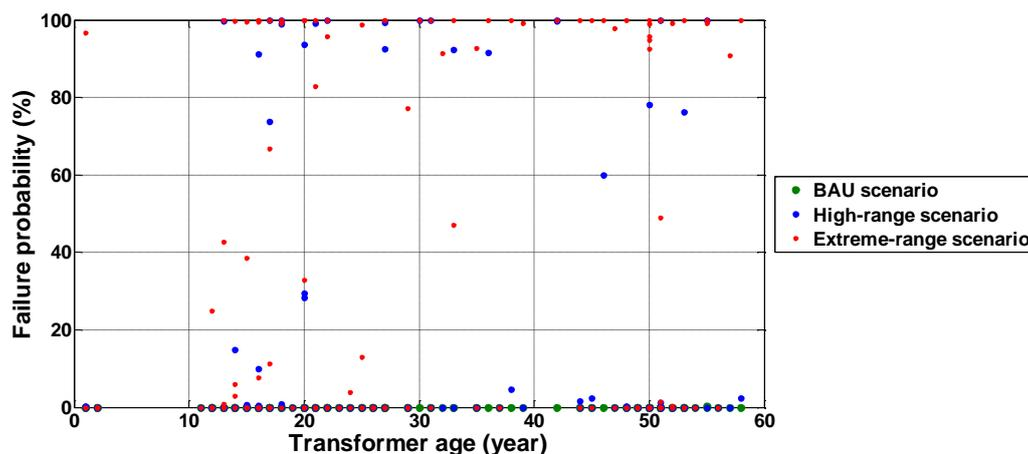
Figure 3.12: Failure probability under three EV scenarios
