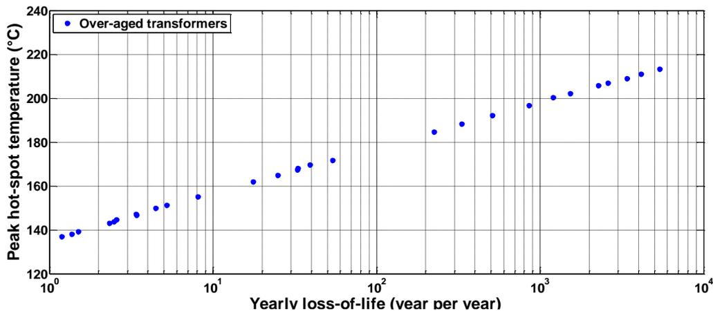
Figure 3.9: Peak hot-spot temperatures of over-aged distribution transformers
