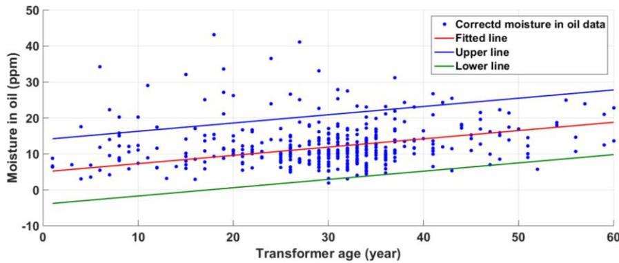
Figure 3.4: Fitting of moisture in oil data of indoor distribution transformers
