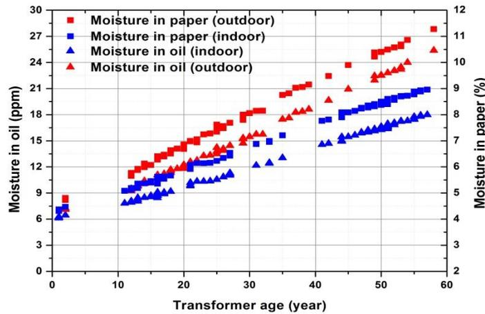
Figure 3.10: Moisture in oil and paper of selected transformers
