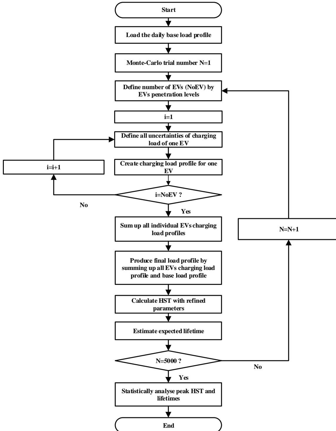
Figure 2.8: Flow chart of Monte-Carlo simulation to determine hot-spot temperature and lifetime of prototype distribution transformer under EV scenarios
