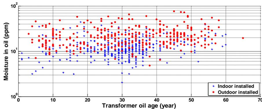
Figure 3.3: Corrected moisture data of indoor and outdoor installed distribution transformers
