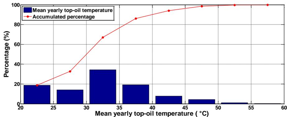
**Figure 3.1: Mean yearly top-oil temperature of distribution transformer population calculated with Elexon profiles**
