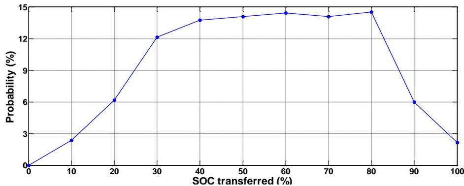
Figure 2.7: SOC transferred in a single charging event [36]
