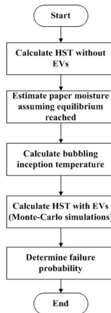
Figure 2.5: Flow chart of modelling failure probability under EV scenarios
