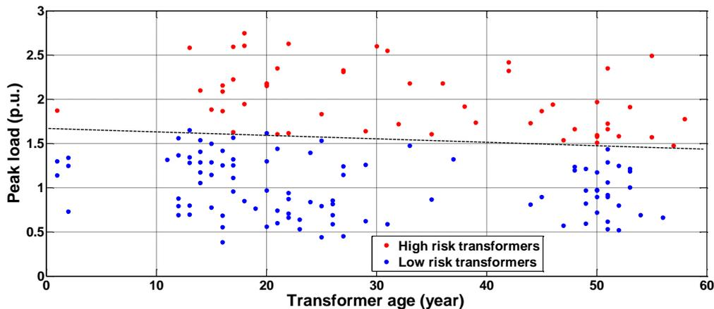
**Figure 3.13: Comparison of peak loads between high risk transformers and low risk transformers under Extreme-range scenario**
