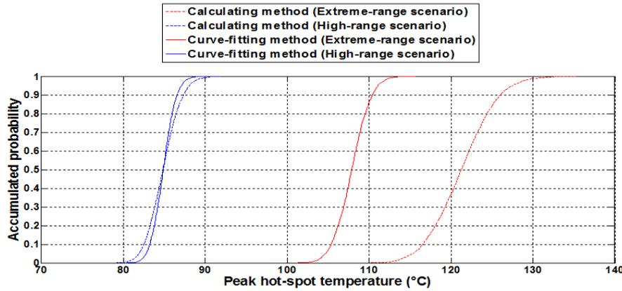
**Figure 2.10: Comparison of CDF of hot-spot temperature under EV scenarios with thermal parameters refined by two methods**
