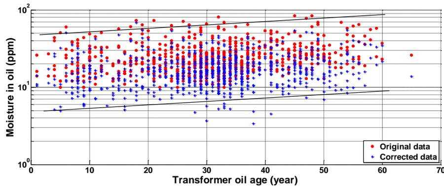
Figure 3.2: Originally measured moisture in oil data and corrected values of distribution transformer population
