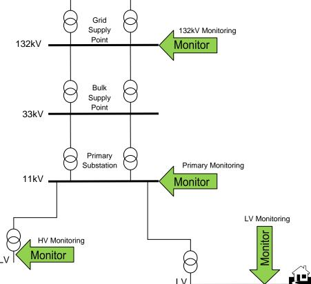
Figure 1: Illustration of CLASS monitoring requirements
