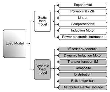
Figure 3.2. Different load modelling techniques [6]
