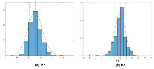
Figure 5.10. Normal distribution of  $K_q$  and  $K_q$  values for 60 monitored substations.
