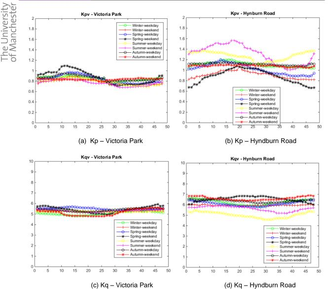
Figure 5.8. Mean values of K<sub>p</sub> and K<sub>q</sub> for mix-type substations: Victoria and Hyndburn Road
