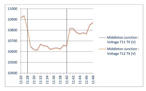
Figure 3 Middleton Junction demand reduction full voltage graph
