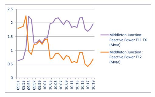
Figure 14 Middleton Junction Stage 1 reactive power absorption effect
