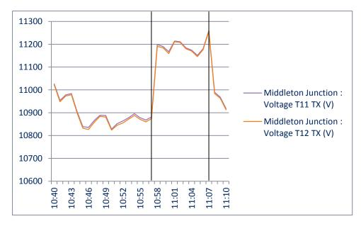
Figure 10 Middleton Junction demand boost half voltage effect
