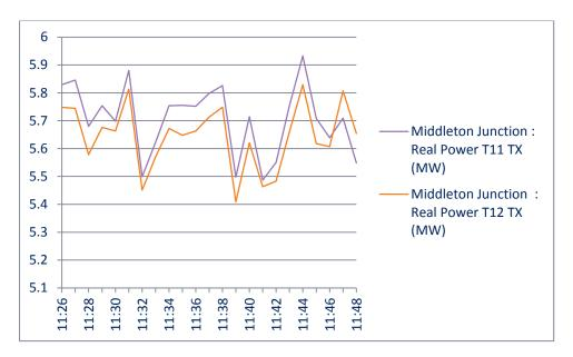
Figure 4 Middleton Junction demand reduction full real power effect
