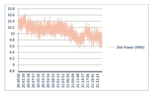
Figure 9 Middleton Junction demand during stage 1 frequency event
