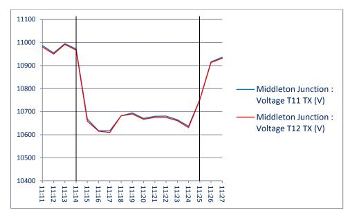
Figure 1 Middleton Junction demand reduction half voltage graph
