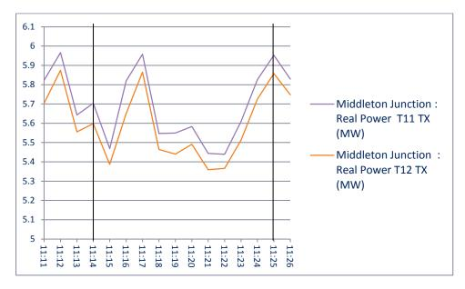
Figure 2 Middleton Junction demand reduction half real power effect
