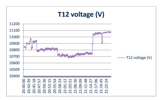
Figure 8 Middleton Junction T12 voltage during Stage 1 frequency response
