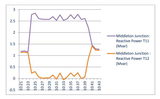
Figure 15 Middleton Junction Stage 2 reactive power absorption effect
