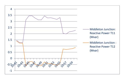
Figure 16 Stage 3 reactive power absorption effect
