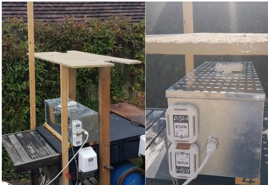
Figure 13: The PMT shade test rig for a simple top canopy, in the initial high position (left), and the later lower position (right), which shows the reduction in sunlight reaching the lid of the box.
