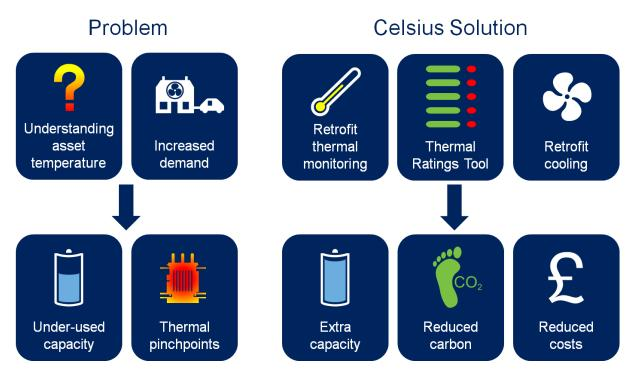
Celsius first seeks to identify potential thermal issues by establishing how different distribution substations in differing environments behave thermally under a variety of load and environmental conditions. Celsius will develop the following methodologies to better understand the real thermal ratings of distribution substation assets in order to unlock capacity:
