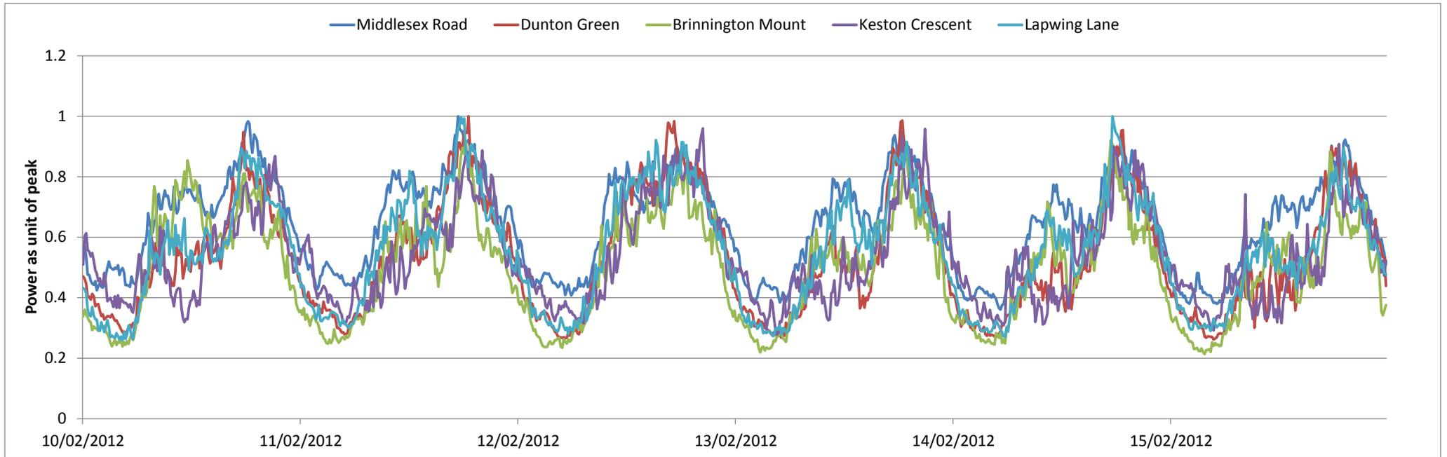
Figure - B-1: Power through all transformers for 10<sup>th</sup>-16<sup>th</sup> February 2012 as unit of peak power
