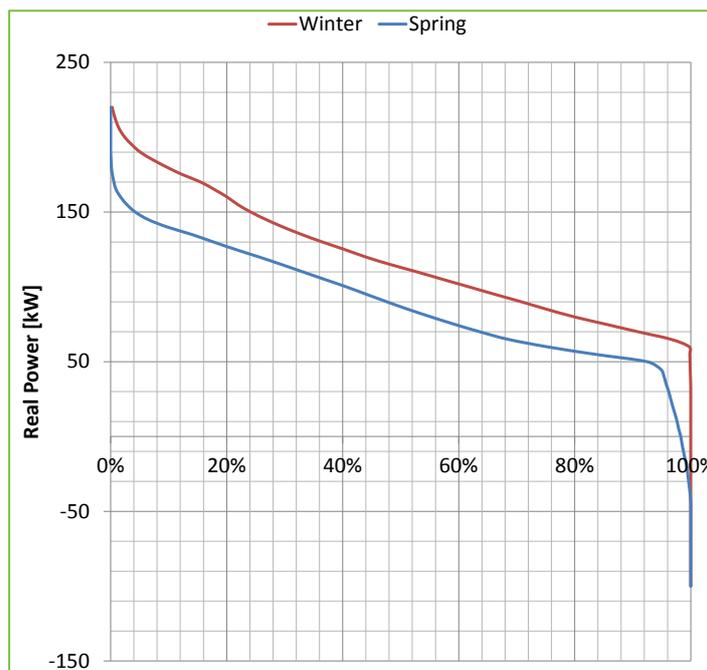
Figure 7-14 - Load duration curve for Dunton Green (all feeders) for winter and spring
