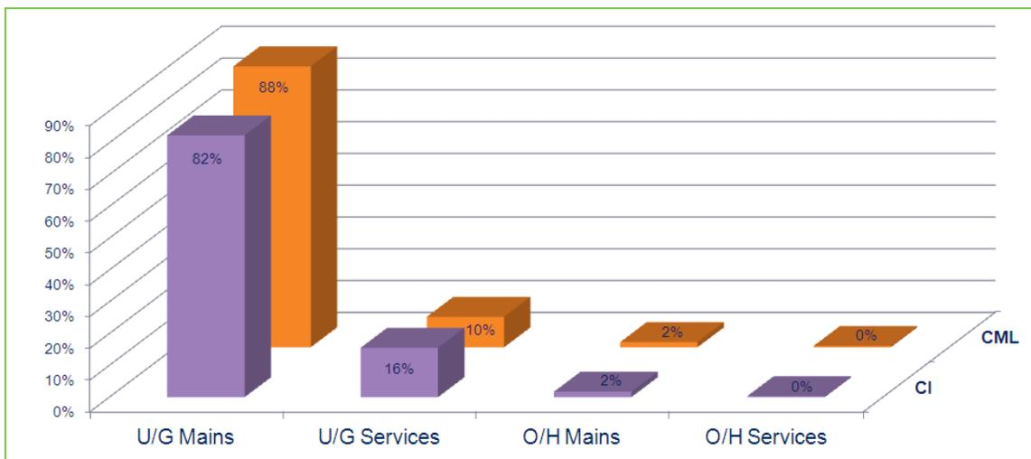
Figure 7-19 – Locations of Transient Faults
