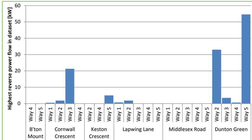
Figure 7-12 - Highest reverse power flow seen on all feeders in the Kelvatek data
