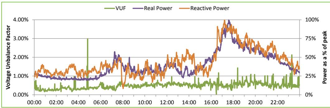
Figure 7-11 - Voltage unbalance factor for single way of Cornwall Crescent, 17th January 2012
