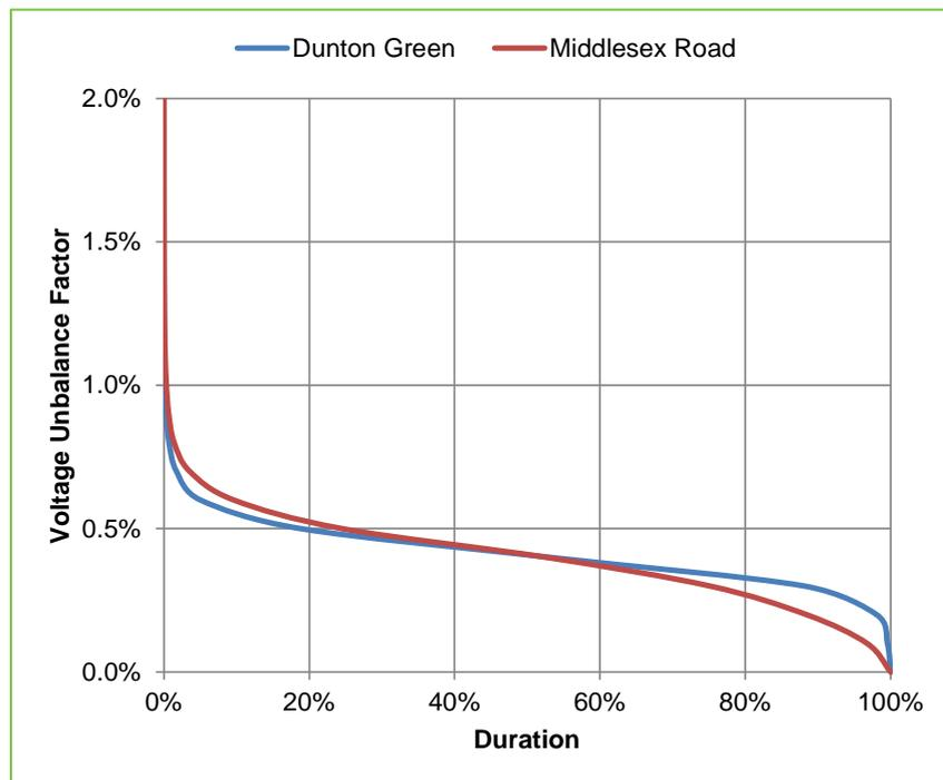
Figure 7-9 - Duration of VUF for Middlesex Road (low PV) and Dunton Green (high PV)
