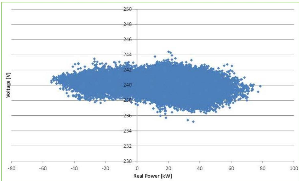
Figure 7-16 - Network voltage and real power flow for Dunton Green, Way 5 which has a high penetration of PV (9th February to 26th June 2012)
