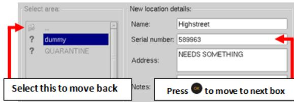
**8** Enter location details. Enter text like basic mobile phone text entry. Press **OK** to change between text entry modes **123** (text, numbers, capitals etc.) Press **OK** to move to between text entry boxes. Name, Serial Number (unique Identifier, e.g. NRN or Substation Code) and Address all require information. When finished choose **Apply**
