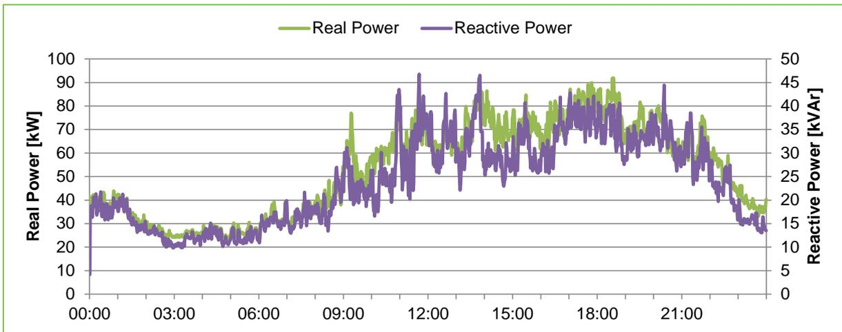
Figure 7-6 - Real and reactive power through Brinnington Mount on 12th February 2012
