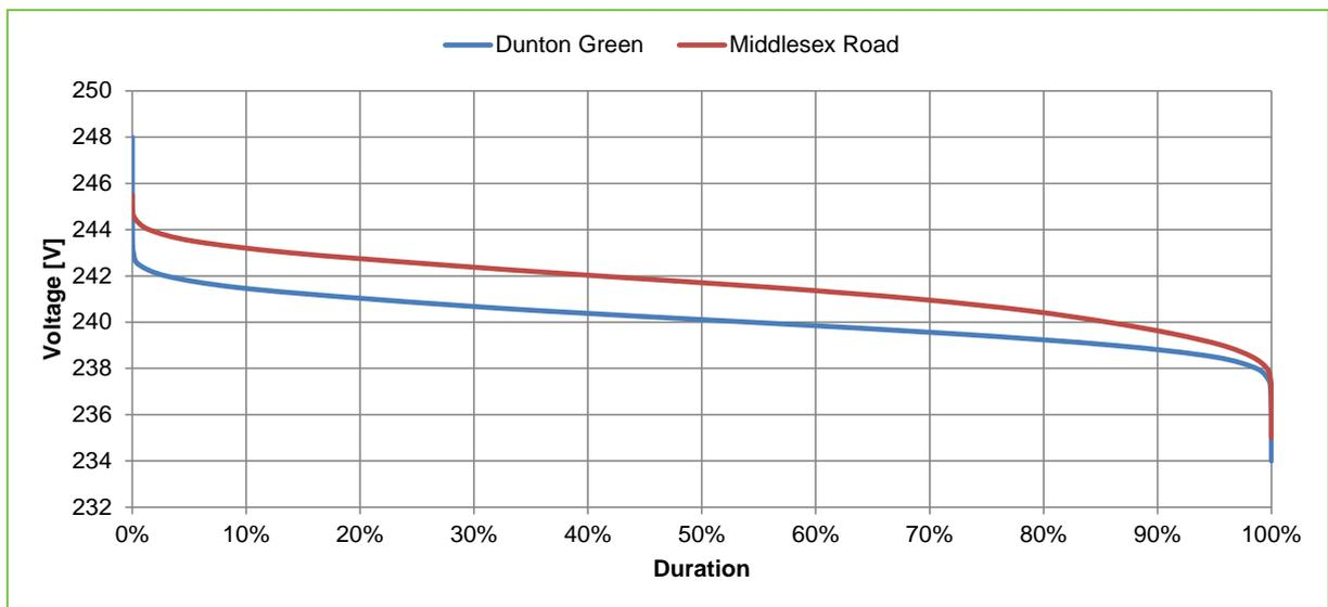
Figure 7-17 - Distribution of voltages for Dunton Green (high PV) vs. Middlesex Road (low PV) for 10/02/2012 to 21/12/2012
