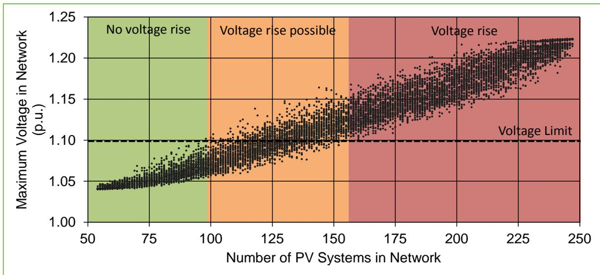
Figure 7-18 - Permissible penetration of PV in an LV network (for illustrative purposes). Here 50,000 load flows are performed with PV at random and feasible locations within the network
