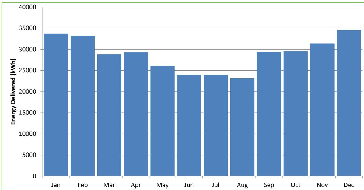
Figure 7-5 - Energy delivered through Keston Crescent transformer in 2012
