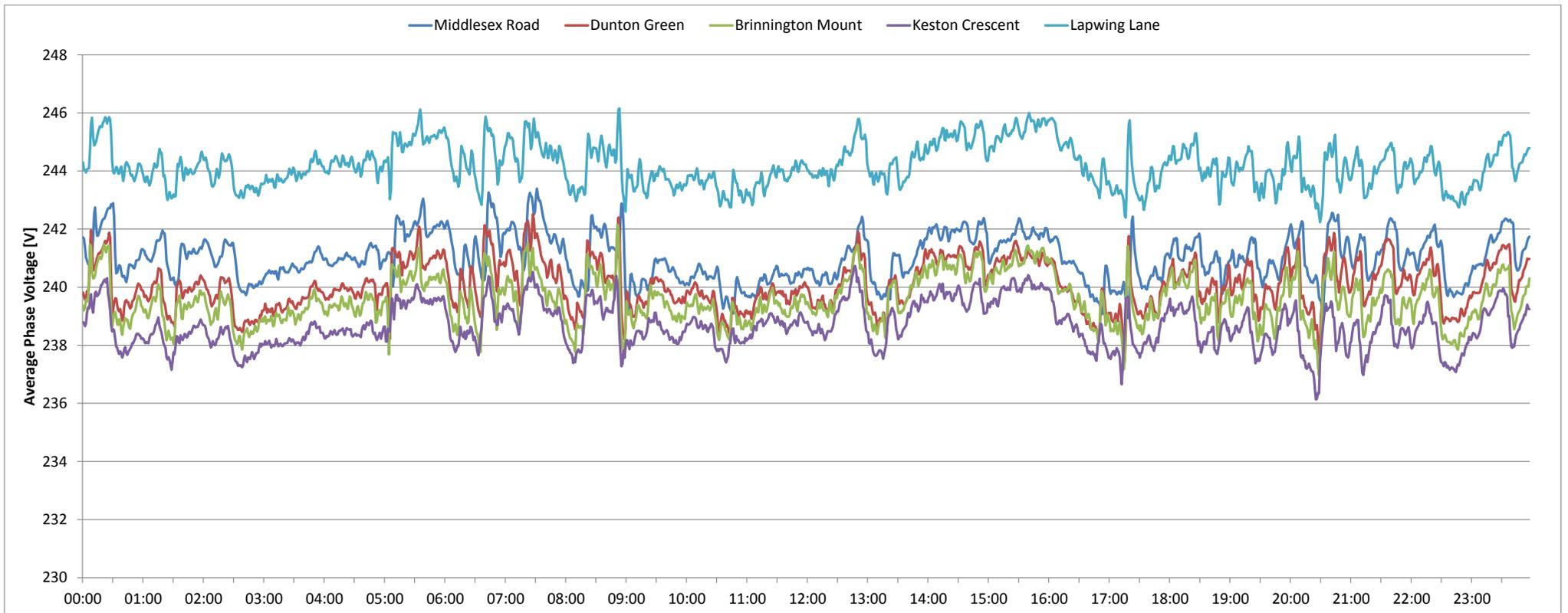
Figure - B-2: Average voltage across phases on 10/02/2012 for all transformers
