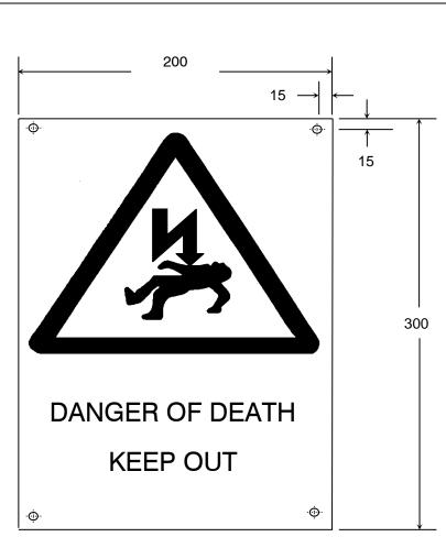
**DIMENSIONS:** FOUR SCREW HOLES = 6mm DIAMETER.
