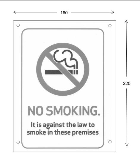
**DIMENSIONS:** FOUR SCREW HOLES, 4mm DIAMETER WITH CENTRES 6mm FROM EACH EDGE.
