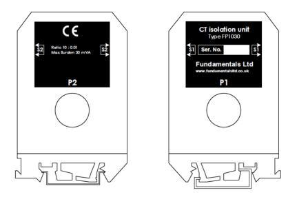
The secondary outputs of this interposing CT will feed into the SuperTapp SG Relay.
