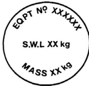
Figure 2 – Detail of marking on end of spindle
