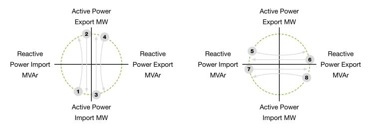
These diagrams assume the other vector (MW or MVAr) does not change during the power swing.
