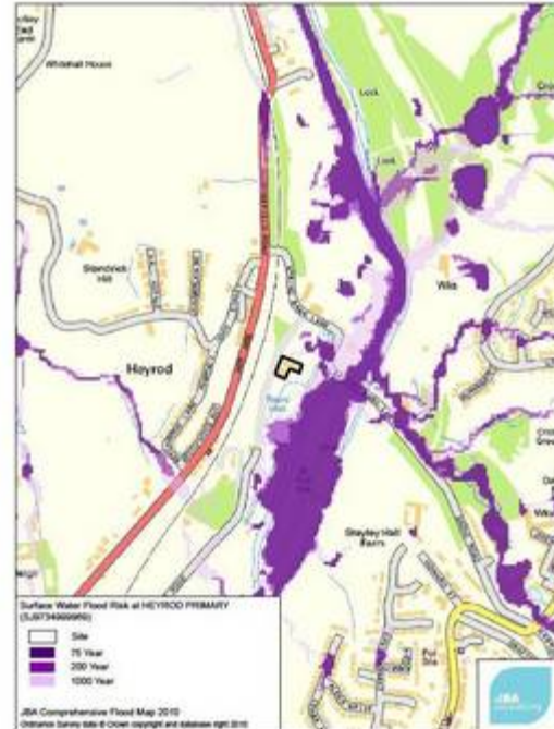
Pluvial flood risk at Heyrod Primary
